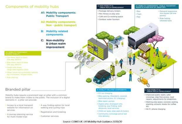
Figure 6.11: Potential Components of a Mobility Hub
