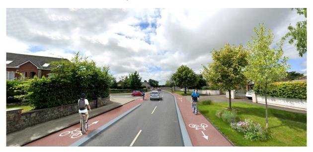
Figure 6.5: Example of Segregated Cycle Route along R659, north of Co-Op Livestock Mart
