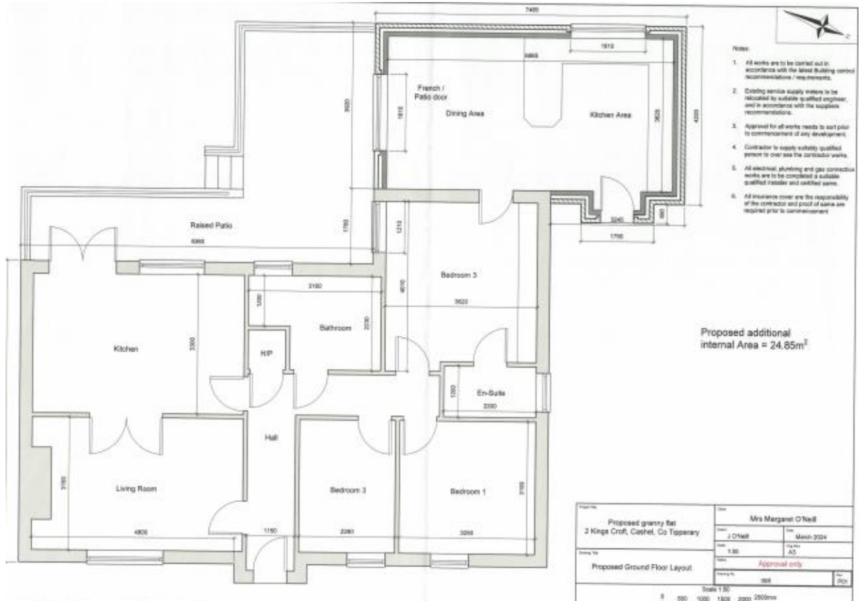
Image 2: Proposed image of Granny Flat to the rear and side of the existing dwelling
